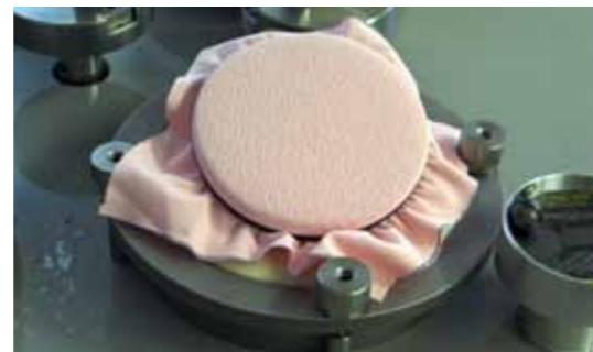
The mechanical stress on textiles is simulated with the "Martindale Abrasion Tester".
