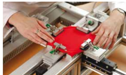
Here the UV protection factor of textiles is also being measured when elongated in a stretching device.
